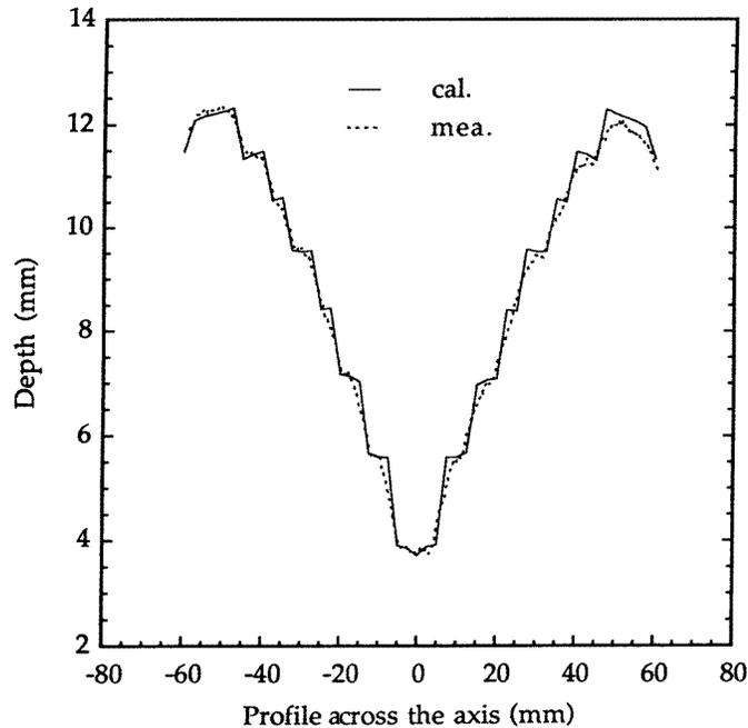
**Figure 2.** The calculated depth (solid line) compared to the milled depth in the Styrofoam block (dashed line) measured with a stylus profiling instrument on a stairlike cross-profile.
