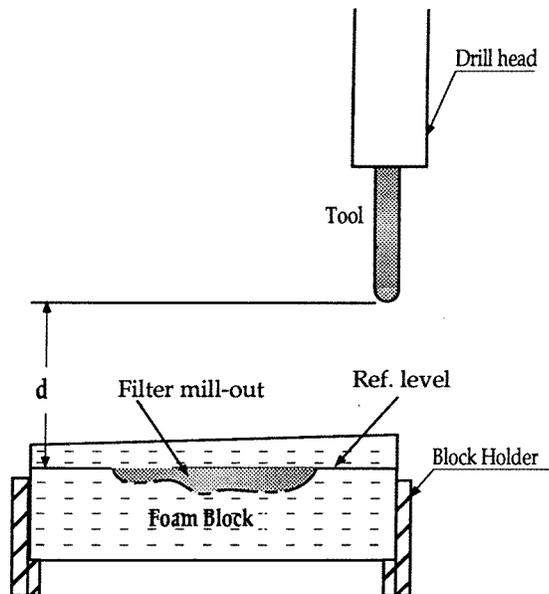
**Figure 1.** A diagram illustrating the geometrical position of the tool tip and the foam block.  $d$  is the distance from the tool tip to the levelled surface (reference level), and it is kept constant over the block surface.
