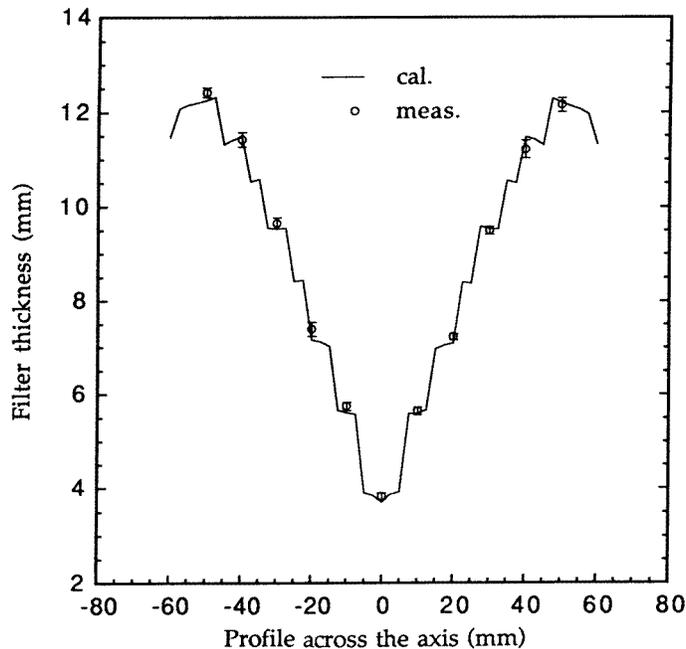
**Figure 3.** The calculated thickness (line) representing a staircase phantom and the measured thickness (symbols with error bars) along a cross-plane of a number of filters. The error bars are the standard deviation ( $1\sigma$ ) from the average thickness of the measured data.
