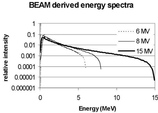
FIG. 2. The energy spectra derived from the BEAM MC code simulations for the Philips SL75/5 (6 MV), Philips SL75/14N (8 MV) and Philips SL25 (15 MV) accelerators. The area under each spectrum is normalized to unity.
