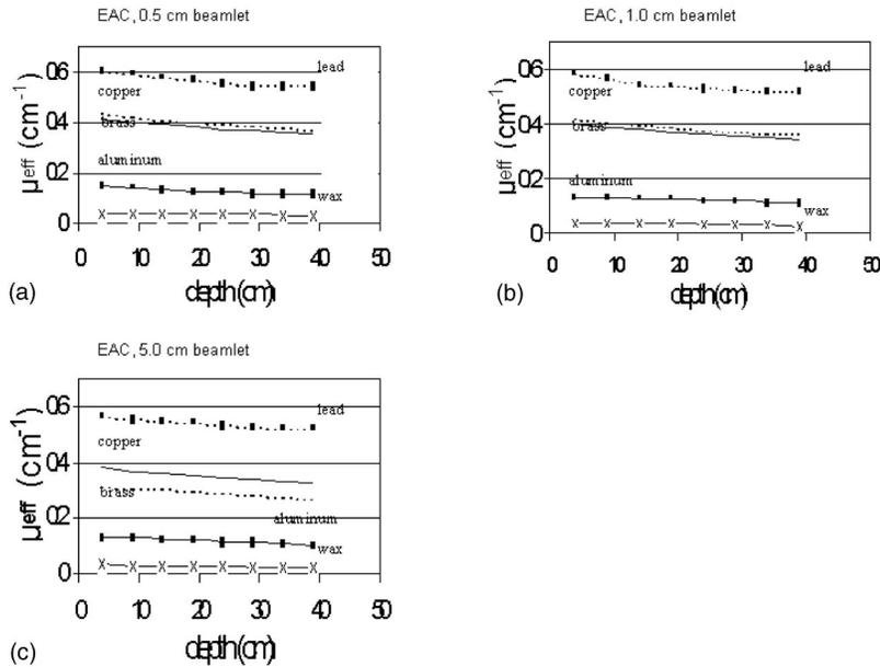
FIG. 6. The dependence of the effective attenuation coefficient on depth for various materials for beamlet areas of 0.5 cm (a), 1.0 cm (b), and 5.0 cm (c) are shown for a 6 MV x-ray beam.
