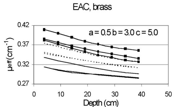
FIG. 5. Effective attenuation coefficients for brass as a function of depth for different beam energies (—■—, 6 MV; ---, 8 MV; and —, 15 MV). Each set of lines corresponds to three different beamlet sizes for the same energy. The smallest beamlet at a given energy has the larger effective attenuation value. Beamlet sizes correspond to 0.5, 3.0, and 5.0 cm side lengths.
