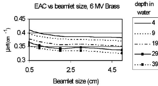
FIG. 4. Effective attenuation coefficients as a function of beamlet area at five constant depths of 4, 9, 19, 29, and 39 cm obtained for brass beam absorbers.
