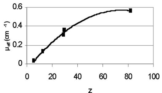
FIG. 7. The dependence of the EAC on the atomic number ( $Z$ ) of the absorber material for a beam energy of 6 MV at a depth of 4 cm. The solid curve represents the fitting equation.
