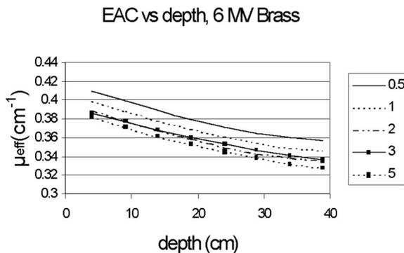
FIG. 3. The effective attenuation coefficient ( $\mu_{\text{eff}}$ ) as a function of depth in water for square beamlet areas with side lengths of 0.5, 1.0, 2.0, 3.0, and 5.0 cm.
