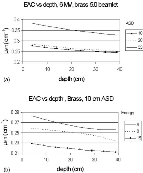
FIG. 8. The variation of the effective attenuation coefficient for brass as a function of depth for 10, 20, and 33 cm absorber-to-skin-distance (ASD) (a) and for 6, 8, and 15 MV beam energies at a ASD of 10 cm (b). In both cases a fixed square beamlet with a side length of 5 cm was used.
